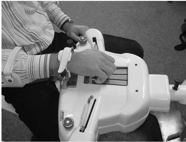
FIGURE 2 Amadeo robotic device with fingers in flexion.
