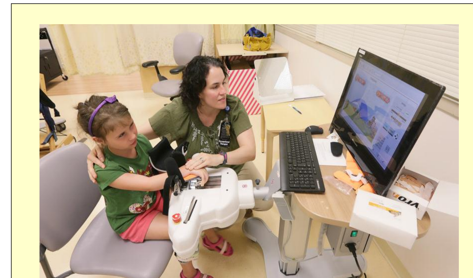
The Tyromotion Amadeo promotes composite or individual digit flexion and/or extension for controlled grasp and release.
