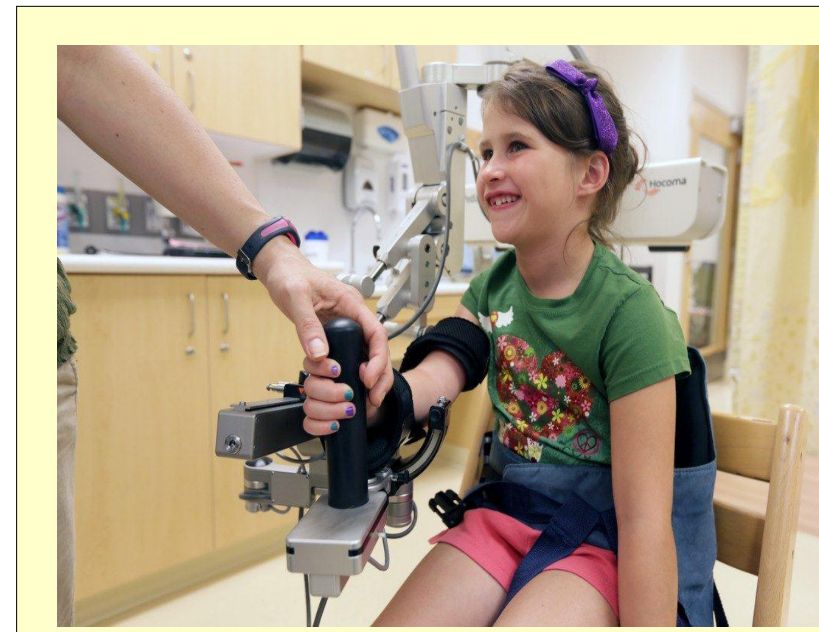
The Hocoma ArneoSpring Pediatric allows for gravity reduced movement of the upper extremity as needed to promote shoulder, elbow and forearm movement and gross grasp and release.
